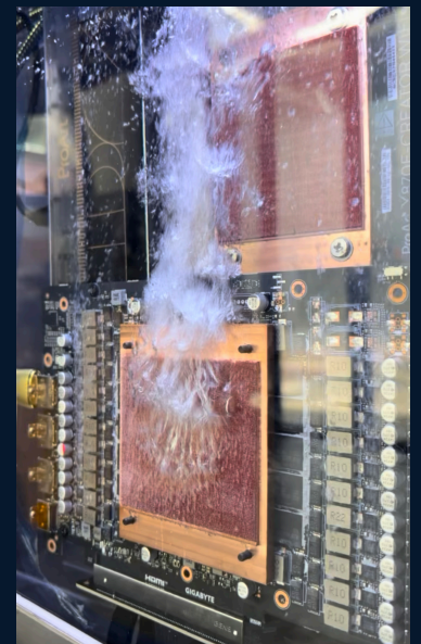
GPU cold-plate immersion-cooling test photograph
